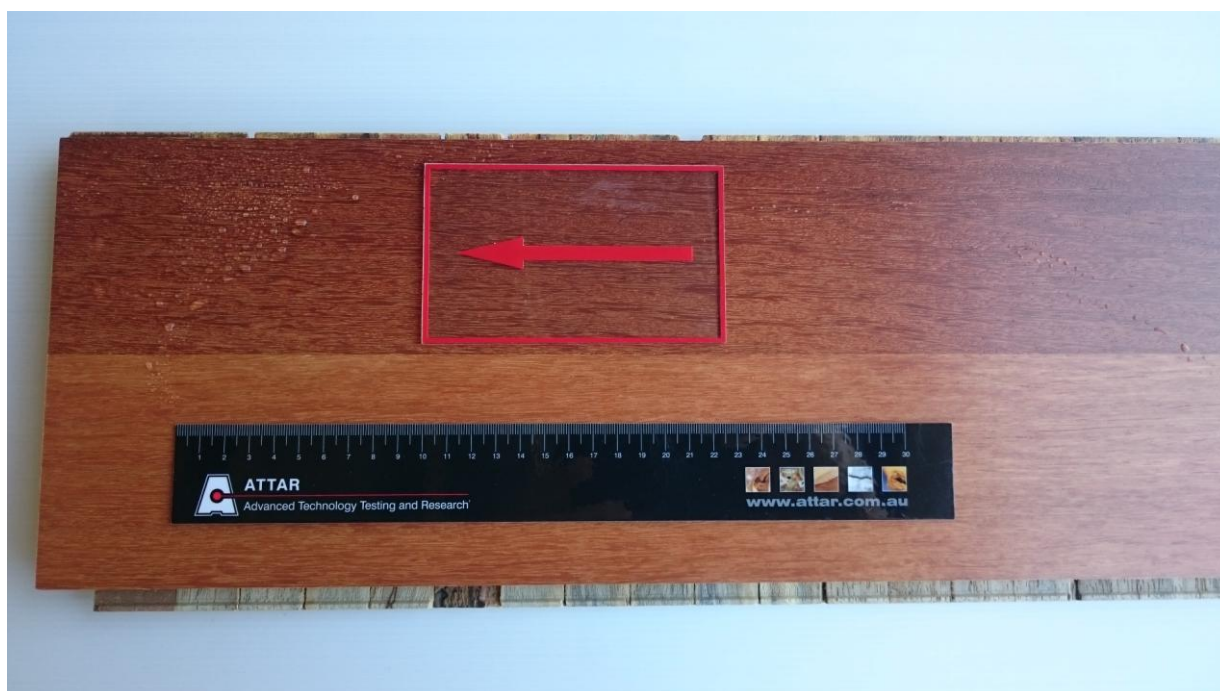
Figure 1: Unilin Engineered wood floor Low Sheen. Highlighted area indicates direction of test.
